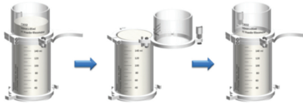
Figure 15 – Vessel splitting is an effective way of generating a precisely known powder volume and a level surface, for the accurate determination of bulk density.
