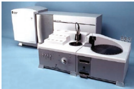
Figure 1. a Beckman Coulter® LS™ Series particle size analyzer, LS 13 320
